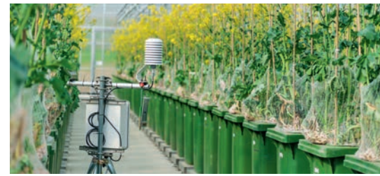
Fig. 19 Digital agriculture: The use of innovative digital methods in the agricultural sciences is a digitalisation priority in research and teaching at JLU. This photo shows the internationally unique DroughtSpotter XXL unit which precisely documents the reactions of over 1,000 plants to drought stress under controlled conditions at five-minute intervals throughout the year.
