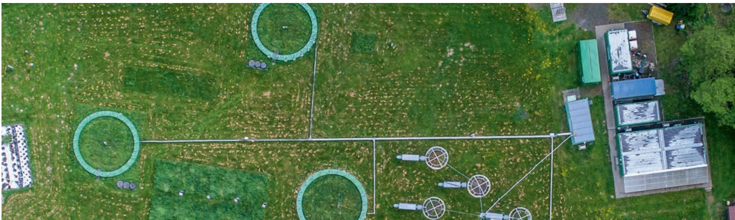
Fig. 20 Research Facility for Climate Effects: To develop strategies to reduce the impact of climate change, the Research Facility for Climate Effects in Linden uses CO 2 enrichment rings to study the effects of carbon dioxide on plants, soil and animals.
